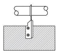
SIZE-SYSTEM PIPE: 3/4" and 1" MATERIAL - Carbon Steel. FINISH - Mil. Galvanized. LISTING/APPROVAL -
