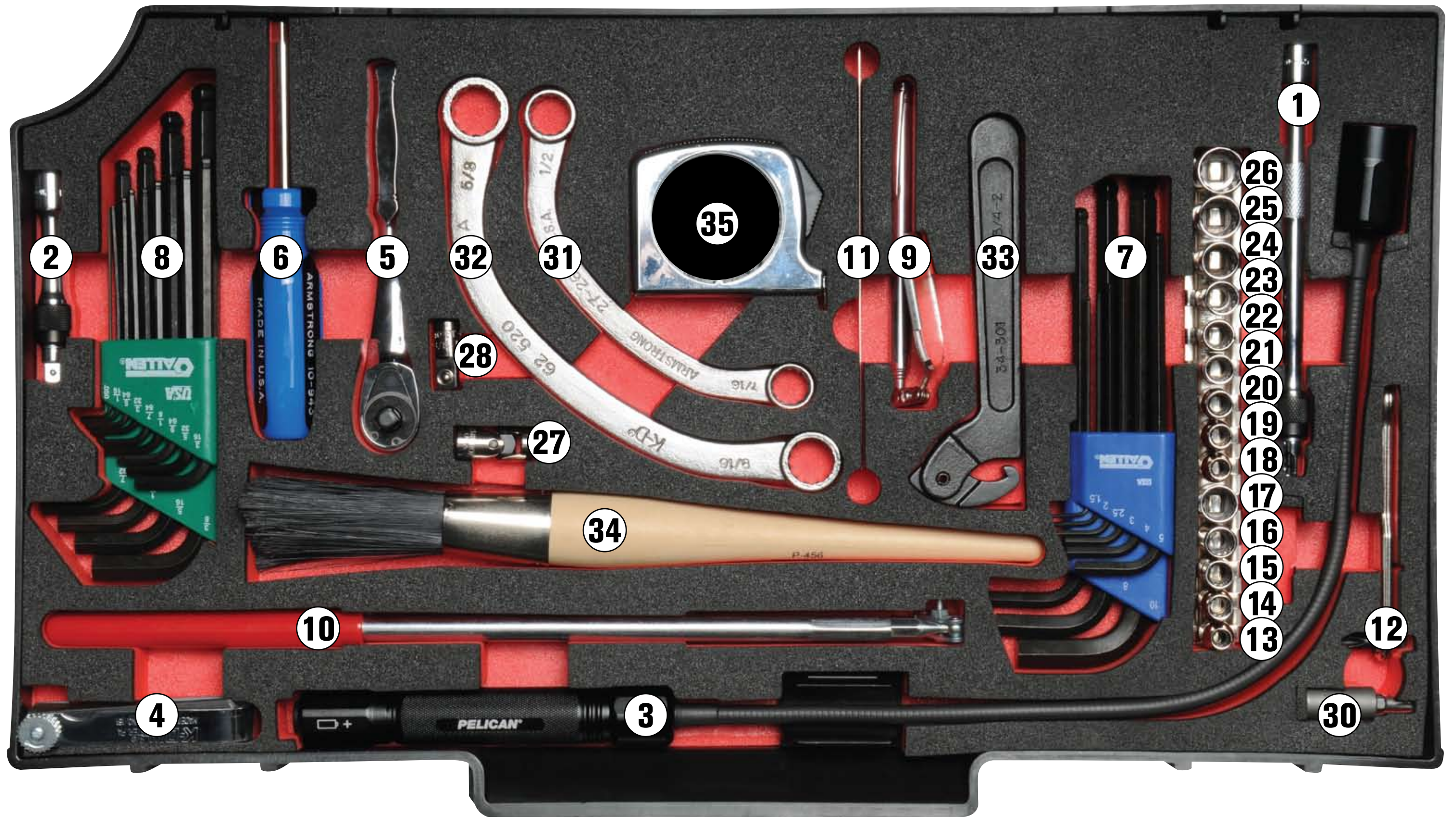
General Maintenance Tool Kit (GMTK) Drawer layout
