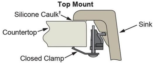
Maximum thickness for use of hold down system is 1-3/4" (44mm).
