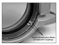
3. CHECK GASKET: Check the gasket to make sure it is suitable for the intended service. Victaulic gaskets for copper products contain two marks: the copper-colored mark identifies that the gasket is specifically for Victaulic copper products, and the additional mark identifies the gasket grade. Refer to submittal 05.01 or the "Gasket Selection" section of this manual for the color code chart.
