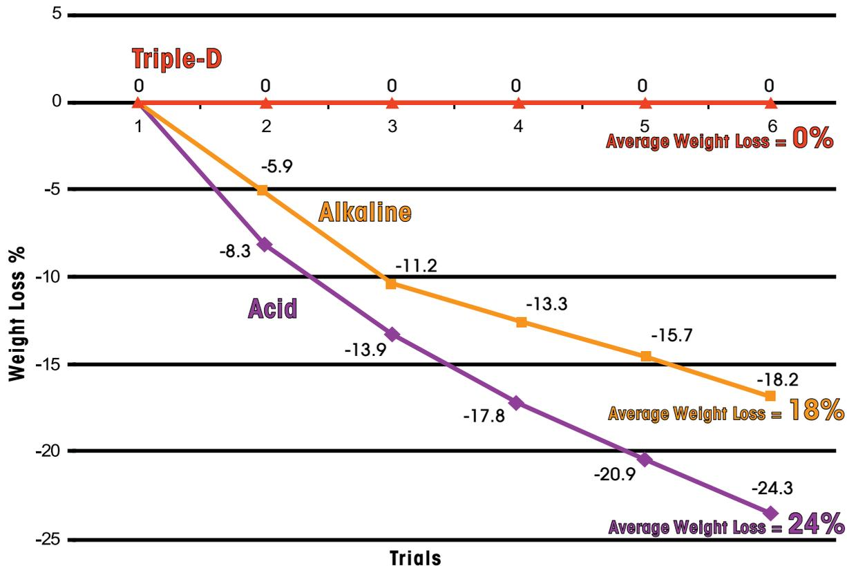
As shown above, conventional foaming acid coil cleaners and foaming non-acid coil cleaners actually attack and chemically react with the aluminum coil components. This reaction is exhibited by a foaming action. The attack/reaction dissolves the aluminum, destroying the heat-transfer ability of the coil creating the potential for refrigerant leaks.
