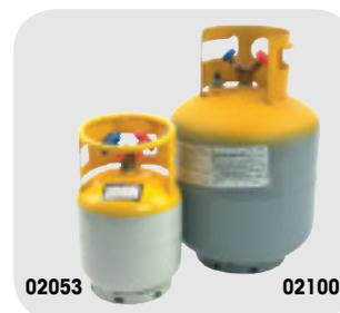
**Caution:** Never overfill cylinders. Maximum refrigerant capacity is limited to 80% of the water capacity of the cylinder in lbs. (see table above). DOT requires cylinders to be retested every five years. Some recovery equipment uses weight scales to cut off refrigerant fill at 80% of capacity. Be sure cylinder tare weight is correct for this type of equipment.
