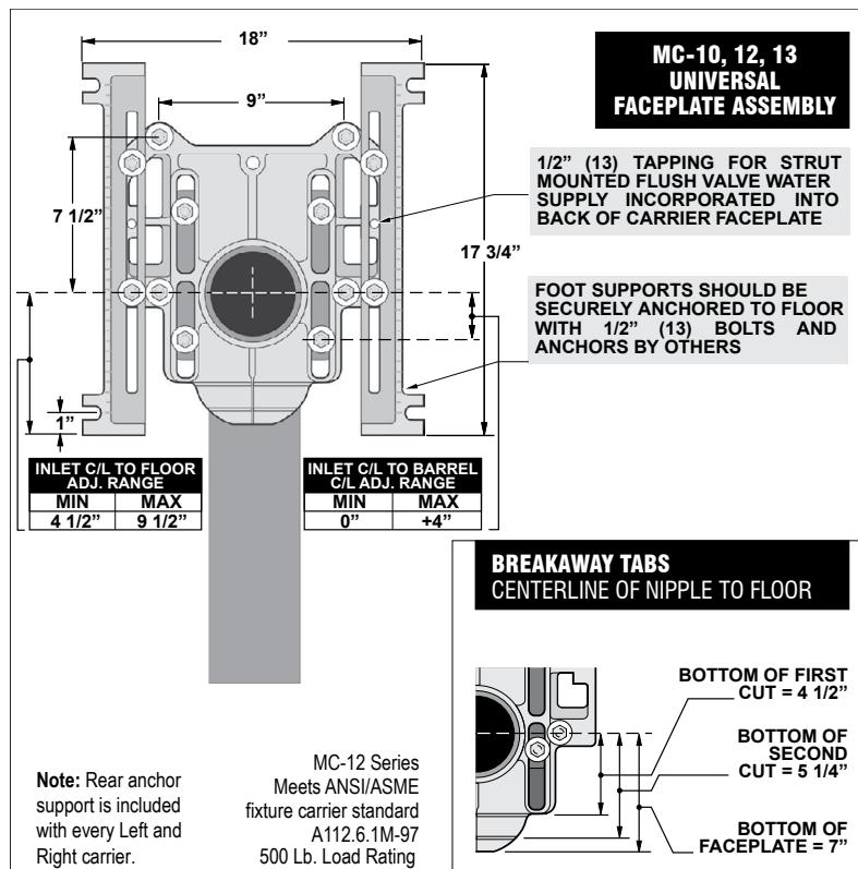
**Note:** 8" tapered thread ABS nipple shipped standard with MC-12 Series carriers. The universal faceplate assembly accepts all nipple variations, rolling thread (-OR), cast iron (-CI) and tapered thread ABS with adjustable horn (-AH).
