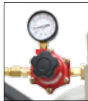
PROPANE REGULATOR VALVE
