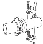
2. Assemble Series 1390 clamping rings onto spigot pipe and just 3. Insert all provided connecting rods and nuts as shown and behind bell end as shown (use restraining rods as a guide to position and align restrainers) and tighten bolts and nuts evenly to at least the minimum recommended torque (see table). A torque wrench is required to ensure proper torque.
