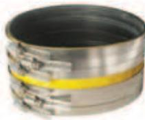
The distinctive yellow shield quickly identifies the Medium-Duty MD Couplings and makes it easier for inspectors. 5/16" hex-head screw applies 80 in.-lbs. of installation torque to the band/shield assembly.
