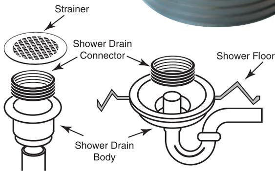
Shower Drain Connectors connect 2" DWV plastic, Sch. 40, steel or X.H. (extra-heavy) cast iron pipe to shower drain bodies. They reduce the time and cost of installation because no special tools, gluing, threading or lead caulking are required.
