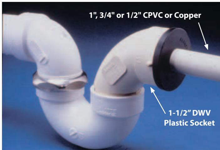
These one piece connectors are designed for quick, easy connections. With a simple press fit (no tools needed) they connect 1", 3/4" or 1/2" CPVC and copper pipe to 1-1/2" DWV Schedule 40 plastic sockets (ABS or PVC).
