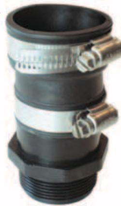
Fernco check valves allow for the unrestricted flow of water up and out through the pipes, but when the pump turns off, the water in the pipes doesn't flow backwards back into the sump pit causing more work and wear on the sump pump.
