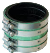
The distinctive green shield quickly identifies the Heavy-Duty HD Couplings and makes it easier for inspectors. 3/8" hex-head screw applies 80 in.-lbs. of installation torque to the band/shield assembly. Boasts an ultimate torque rating exceeding 100 in.-lbs. and heavier gauge stainless steel.
