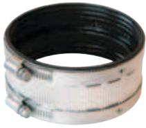
5/16" hex-head screw applies 60 in.-lbs. of installation torque to the band/shield assembly.
