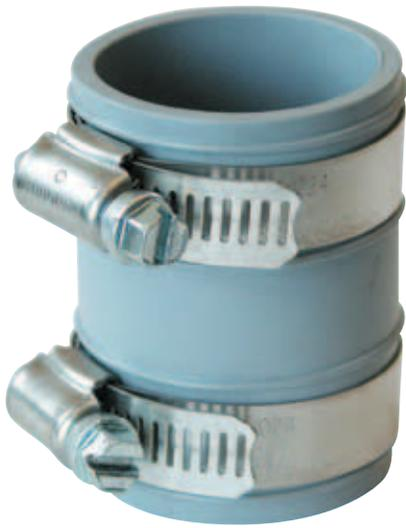
Fernco Tubular Drain Pipe Connectors offer a quick, easy way to extend, alter or repair any combination of 1-1/2" or 1-1/4" (32 or 38mm) brass or plastic drain pipe. Whether you're connecting brass to brass, plastic to plastic, or brass to plastic, you get an economical, leak free seal. Installation is fast and simple. The flexible elastomeric PVC material is formulated for drain use and provides a strong, reliable connection that's made in minutes, but lasts for years.
