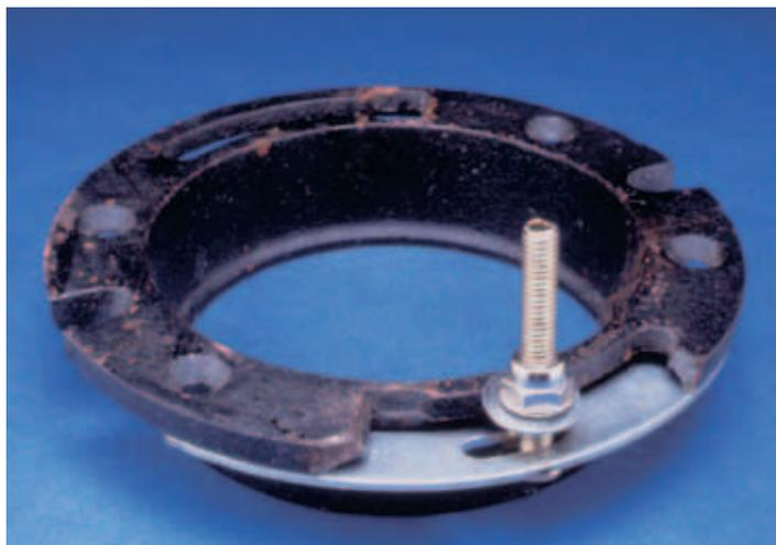
FIX-A-FLANGE eliminates the need to replace broken toilet flanges, saving time and money. Simply place the flange under the broken area of the ring and tighten the nut.
