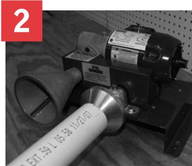
Chamfer (bevel) the end of the pipe  $10^{\circ}$  -  $15^{\circ}$ .
