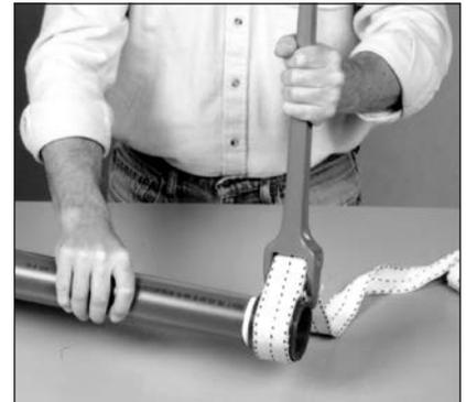
**NOTE:** Threading of PVC Schedule 40 and CPVC Schedule 80 pipe is not recommended. Threading pipe over 4" in diameter is not recommended.
