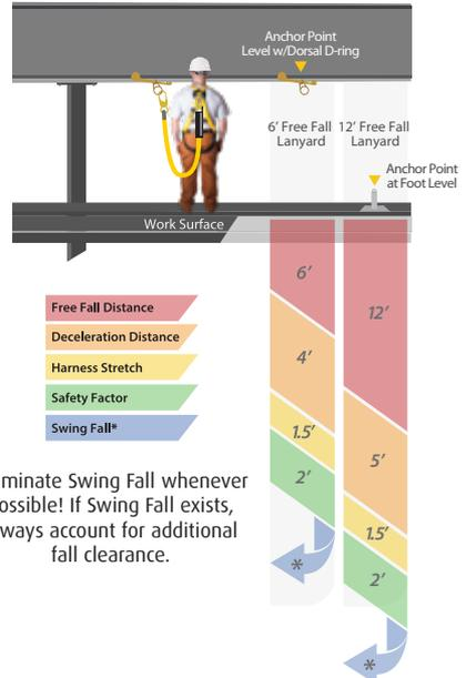
\*Eliminate Swing Fall whenever possible! If Swing Fall exists, always account for additional fall clearance.
