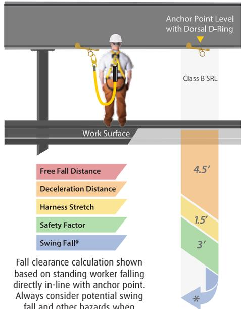
Fall clearance calculation shown based on standing worker falling directly in-line with anchor point. Always consider potential swing fall and other hazards when calculating fall clearance.
