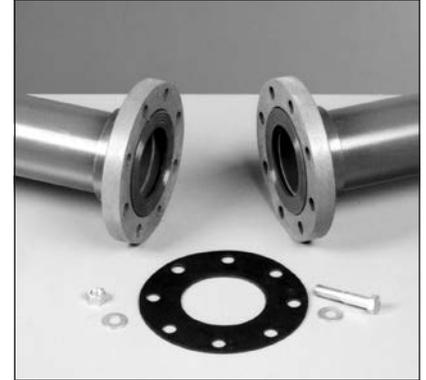
2. Use a full faced elastomeric gasket which is resistant to the chemicals being conveyed in the piping system. A gasket 1/8" thick with a Durometer, scale "A", hardness of 55 -80 is normally satisfactory.
