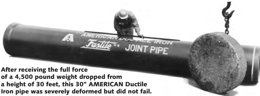
**After receiving the full force of a 4,500 pound weight dropped from a height of 30 feet, this 30" AMERICAN Ductile Iron pipe was severely deformed but did not fail.**
