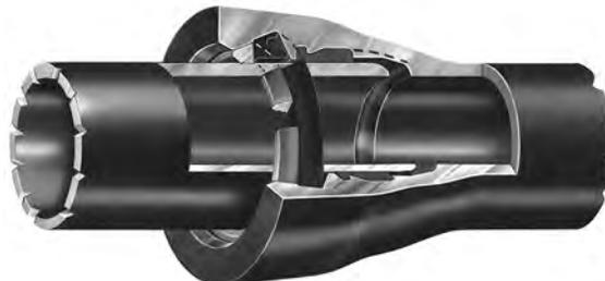
The AMERICAN Field Flex-Ring provides dependable field-adaptable restraint against thrust due to external forces or internal water working pressure up to 350 psi for 14"-24" sizes and up to 250 psi for the 30"-36" sizes in the standard Flex-Ring Joint.
