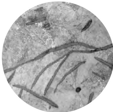
Photomicrograph showing graphite form in gray iron.
