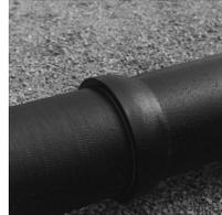
If the joint is to be deflected less than 2 1/4° for 20", 1 3/4° for 24", and 1° for 30", simply push the pipe spigot until it contacts the back of the socket and deflect. If the joint is to be deflected greater than these amounts, push the pipe spigot into the bell (while in straight alignment) only until the leading edge of the factory-applied yellow assembly stripe is even with the face of the bell. The desired deflection up to the maximum may then be set.
