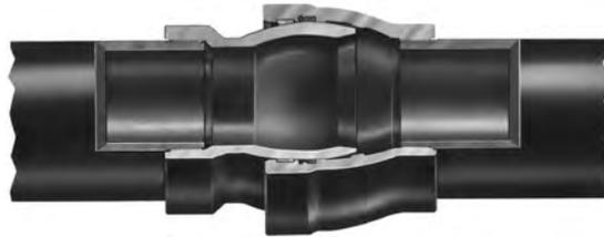
The AMERICAN Flex-Lok Joint, furnished in sizes 30" through 60"\* , is a superservice, boltless flexible joint. This joint is designed to provide up to 15° joint deflection for subaqueous or other difficult installations potentially subject to substantial joint deflections or movements. \*See page 10-2 and check AMERICAN 64" requirements.
