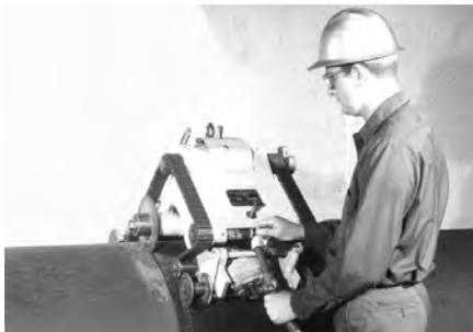
**Cutting ductile iron pipe with milling cutter.**
