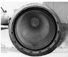
in the ring opposite the bulge. The ring may then be allowed to slide circumferentially around the socket toward the loop, thus relieving rubber compression in the bulging area. Make sure that the angled bearing surface of the segments are secure against the socket, and the toothed side of the segments are facing inward. This should be done by examining and pushing each segment toward the back of the socket until the rubber backing ring is firmly in place against the socket centering throat.
