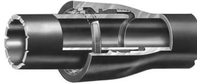
AMERICAN Field FLEX-RING® Spigot Rings are intended for use with AMERICAN Flex-Ring® Ductile Iron Pipe, 6-, 8- and 12-inch, for thickness classes 53 through 56 per ANSI/AWWA C151/A21.51 having a pressure rating of 350 psi.
