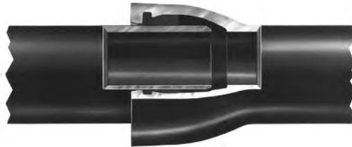
The AMERICAN Fastite Joint, furnished in sizes 4"-64", is a flexible, rubber ring compression-type joint used extensively in underground service. See pages 2-6 through 2-15 and Sections 3, 4, 7 and 9.
