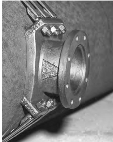
Outlet/Tapping Saddles provide an effective, field adaptable, and economical means of making connection to a pipeline, either during construction or while under pressure. Saddles are available with flanged or mechanical joint outlet for use on pipe sizes 16" through 54". See Section 7.
