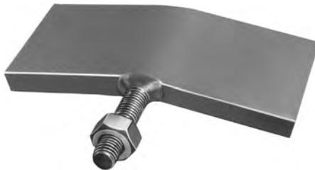
A steel wedge with a welded-on threaded stud, as shown above, is provided for each 4"-24" AMERICAN Flex-Lok joint. One wedge is placed into the space between two lugs and bolted into position. This wedge provides a positive lock to prevent gland rotation after assembly.
