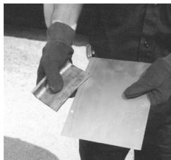
B) Using gloves to protect hands from sharp edges, insert the long end of a disassembly shim fully into the groove in the shim holder. Two lengths of shims are supplied with the 18"-36" disassembly kit for customer convenience. The shorter shims may often be easier to use in some hard-to-reach locations such as the bottom of a joint, or when a small gap exists between the longer shims.
