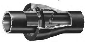
The AMERICAN Field Flex-Ring provides dependable field-adaptable restraint against thrust due to external forces or internal water working pressure up to 350 psi for 14"-24" sizes and up to 250 psi for the 30"-36" sizes in the standard Flex-Ring Joint.
