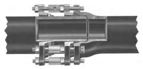
The AMERICAN MJ Coupled Joint is furnished in sizes 4" through 48" and is an adaptation of the standard Mechanical Joint to provide joint restraint against thrust due to internal pressure up to 350 psi through 12" and 250 psi for 14"-48" sizes. See Section 9.
