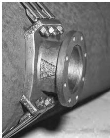
Outlet/Tapping Saddles provide an effective, field adaptable, and economical means of making connection to a pipeline, either during construction or while under pressure. Saddles are available with flanged or mechanical joint outlet for use on pipe sizes 16" through 54". See Section 7.
