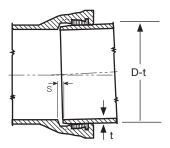
Maximum allowable separation, "S", in a push-on fitting joint is approximately equal to the median pipe diameter in inches times the sine of the deflection angle. This is provided for information only and should not be used to determine precise joint deflection.
