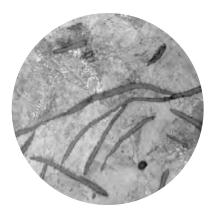
Photomicrograph showing graphite form in gray iron.
