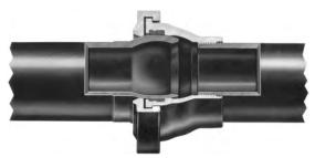
The AMERICAN Flex-Lok Joint, furnished in sizes 4" through 24", is a super-service, boltless flexible joint. This joint is designed to provide up to 15° joint deflection for subaqueous or other difficult installations potentially subject to substantial joint deflections or movements.
