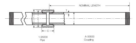
AMERICAN Ductile Iron Threaded Joint Pipe offered several advantages over other pipe materials, namely, long life, uniformity of product, high physical strength properties, and easy threading.
