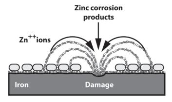
Zinc is anodic to iron. That means iron is the more stable, more noble, of the two elements. Zinc will cathodically protect the iron pipe as long as zinc is present, and over time, will convert to zinc compounds that provide an enduring passivating layer under the topcoat, which protects the pipe against further corrosive attack. Zinc is an anode, uniformly adhered to the surface of the pipe.
