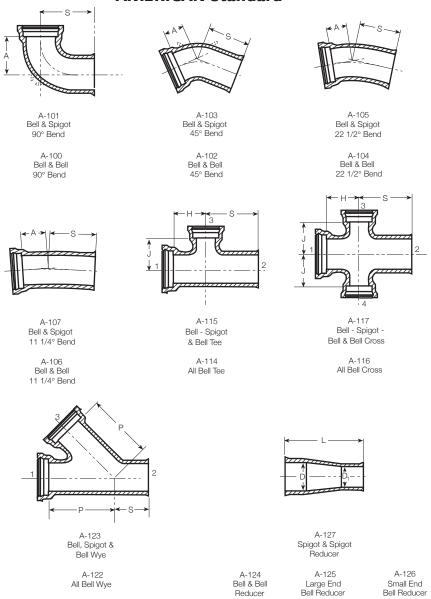
AMERICAN furnished a complete line of Short Body Bell and Spigot Fittings per ANSI A21.10 and AMERICAN Standard as shown above. Bell and Bell as well as Bell and Spigot Fittings (including Spigot and Spigot Reducers) were furnished. The laying length dimensions and "R" dimensions were the same as those of the corresponding mechanical joint and flange fittings per AWWA C110. See Sections 5 and 6.
