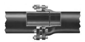
The AMERICAN Mechanical Joint, furnished in pipe sizes 4"-12" and in fittings sizes 4"-48", is a flexible stuffing box type connection used primarily in underground service.
