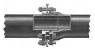
Mechanical Joint Retainer Glands—for use with Ductile Iron pipe 3" through 24"—are cast of Ductile Iron, Grade 60-42-10, and equipped with special alloy steel cupped end set screws. They provide restraint against possible separation of unblocked joints due to internal pressure when assembled on AMERICAN Mechanical Joint Pipe or fittings or on other Standardized Mechanical Joints.
