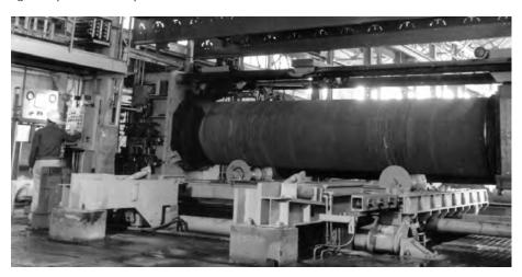
Each 30" and larger diameter AMERICAN Ductile Iron pipe is hydrostatically tested to 75% of yield strength which results in higher test pressures than those required by AWWA C151, varying to over 900 psi, depending on size and thickness of the pipe.
