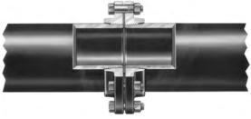
The AMERICAN Flanged Joint, furnished in sizes 4" through 64", is a rigid joint widely used for exposed plant piping. In combination with other joints and AMERICAN's Toruseal® gasket, it is also commonly used for Long Span service.
