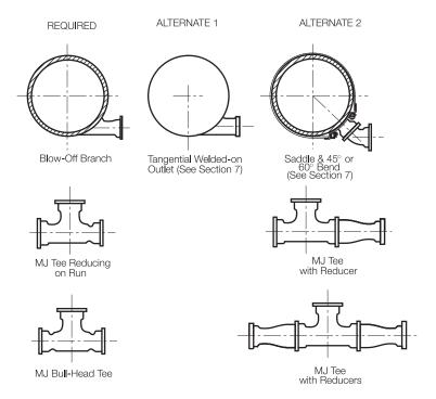
In many cases special fittings for various conditions are required; some of these are shown above in columns headed "Formerly Required." Under the columns headed "Preferred Alternate" are shown combinations of standard fittings which in some situations will provide the desired connection. For economy and availability, it is often advantageous to use the standard fittings.
