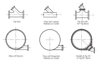
In many cases, special fittings for various conditions are required. Some of the more common of these are shown above in columns headed "Required." Under the columns headed "Alternate," are shown combinations of standard fittings that in some situations will provide the desired connection. For economy and/or shipment from stock, it is often advantageous to use the standard fittings.
