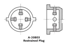
The Fastite Restrained Plug provides positive locking against joint separation and allows for future removal. This plug is also useful as a test plug.
