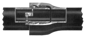
The AMERICAN Lok-Ring® Joint is another restrained joint that utilizes the sealing features of the time-proven AMERICAN Fastite Joint. It is an essentially boltless, flexible restrained connection that provides an easily assembled positive restraint against endwise separation due to thrust resulting from internal pressure or external forces. Only a minimal amount of time is required to complete the Lok-Ring assembly, or disassembly if necessary.
