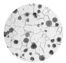
Photomicrograph showing graphite form in ductile iron.
