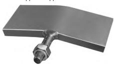
A steel wedge with a welded-on threaded stud, as shown above, is provided for each 4"-24" AMERICAN Flex-Lok joint. One wedge is placed into the space between two lugs and bolted into position. This wedge provides a positive lock to prevent gland rotation after assembly.
