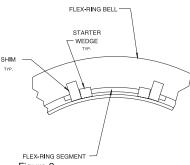
Figure 2 Shim and wedge arrangement for 16", 24", 30", 42", 48", and 54" sizes.
