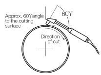
Torch cutting ductile iron pipe Fig. 3-3
