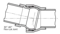
Cross-sectional view showing the AMERICAN Flex-Lok Joints in the deflected position. Note that the waterway remains unobstructed when the joint is fully deflected.
