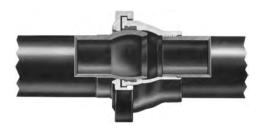
The AMERICAN Flex-Lok Joint, furnished in sizes 4"-24", is a boltless, very flexible joint. This joint is designed to provide up to  $15^{\circ}$  joint deflection for subaqueous or other difficult installations.
