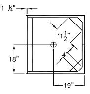
G 3679 SH 3P GELCOAT SECTIONAL SHOWER. UNIT HAS MOLDED CORNER SOAP DISHES, AND CENTER DRAIN LOCATION. UNIT COMPLIES WITH ANSI Z124.1-2, NAHB, AND UPC.
