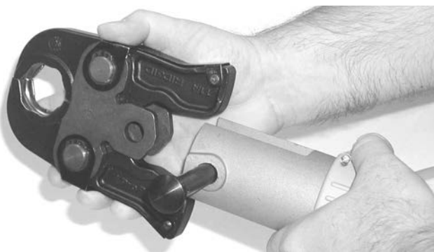
Figure 5 – Pulling The Jaw Set Mounting Pin Out
