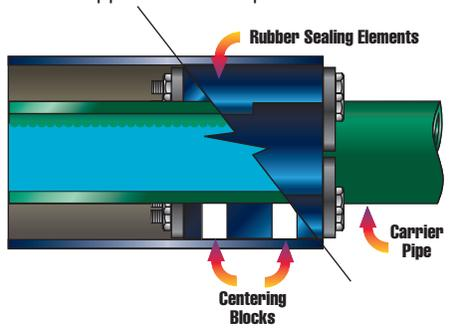
\*Centering Blocks are plastic reinforcements that assure a penetrating pipe will stay "centered" within its casing and adds extra support against heavy loads from back fill.
