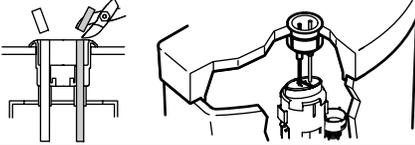
**21** Press the large button onto the black rod. Press the small button onto the green rod.
