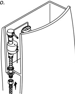
**8** Slide nut onto the supply hose, with flared end last and run hose through toilet wall.
