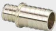
Viega PureFlow Crimp adapter Zero Lead - Brass - Crimp connection, polyethylene (PE) connection Note Use standard stainless steel hose clamp for PE connection (not included) Model V5047ZL
