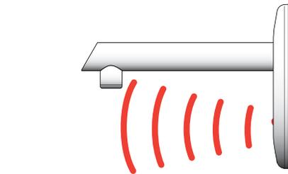
2. As the user's hands enter the beam's effective range, the beam is reflected back into the sensor receiver and activates the solenoid valve allowing tempered water to flow from the faucet. Water will flow until the hands are removed or until the faucet reaches its automatic time out limit setting.
