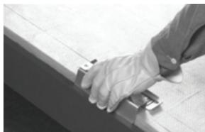
3. Use orange tool to cut right and left hand shi laps for folding duct. Start with right hand groove, turn tool around for second (left hand) groove, turn back to cut third (right hand) groove. (Use red tool for all 3 V-grooves.)
