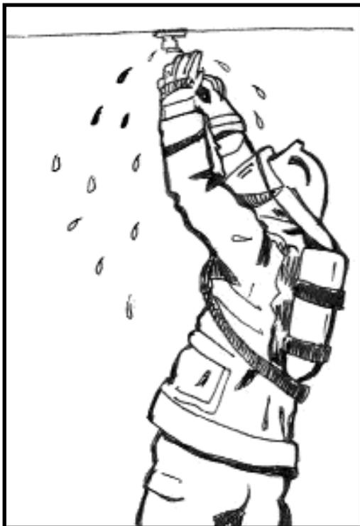
Simply push rubber stop into opening of sprinkler head and turn handle until water flow stops.
