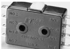
Double-pole double-throw (DPDT) switches are available for isolation of two circuits operating at the same time. One DPDT operates identically to two SPDT being actuated simultaneously. Electrical Ratings 4.5 A at 250 VAC
