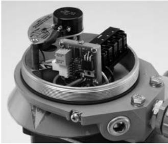
The Quartz two-wire 4-20 mA position transmitter offers exceptional accuracy, reliability and performance. It may be directly attached to positioners or actuators in both linear and quarter-turn applications. You can select either standard or high-performance versions. Span Range: 35° to 270° (Adjustable)
