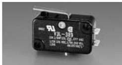
Mechanical (SPDT) standard silver contact micro switches are ideal for high power applications and gold contacts for 24 VDC low power applications. Temperature range -40...+80 °C / -40...+176 °F
