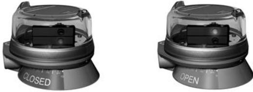
Coordinated visual indicator and LEDs give you an extra measure of safety and increased convenience during plant start-up and operation. Green visual indication and green LED means the valve is open and the control circuit is properly operating. Red visual indication and red LED means the valve is closed and the control is properly matched.
