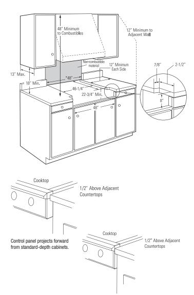
Front of deep cabinets can align with control panel beveled edge.
