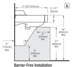
Note: All dimensions and specifications are nominal and may vary: Dimensions of 8" and greater have a tolerance of +3%. Dimensions less than 8" have a tolerance of +5%. Please utilize the current cutout template for countertop cutouts.
