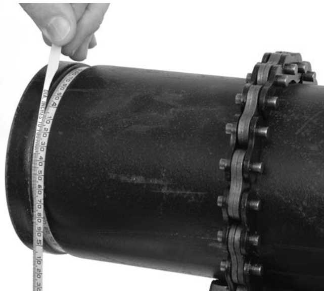
Figure 11 – Checking Groove Diameter With A Diameter Tape
