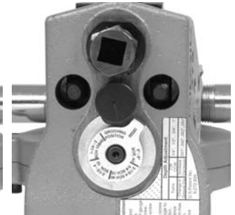
Figure 15B – Gauge In Grooving Position
