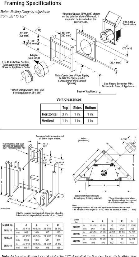
*Note:* All framing dimensions calculated for 1/2" drywall at the fireplace face. If sheathing the chase or finishing with other thickness materials, calculations will need to be made.
