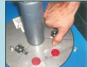
To access controller, flip thumb clips and remove small plate
