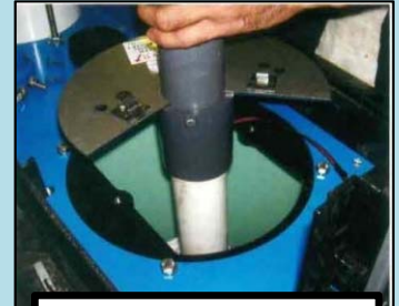
Pull up on inner piping
