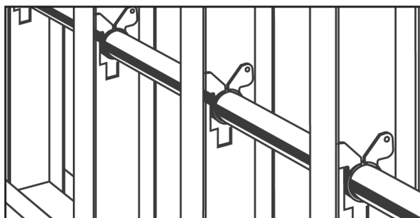
Figure 9.5 Suspension clip fasteners used to protect tubing from abrasion when passing through steel studs
