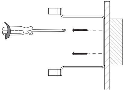
**Note:** If not mounting directly into a wood structure use appropriate hardware capable of supporting item.
