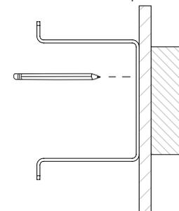
7 Secure Bracket to wood structure (i.e. wall stud) or similar using the supplied screws.
