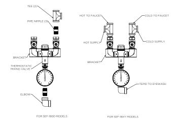
(2) bushings, (1) reducing nipple, (1) adapter, and (3) hoses are not shown
