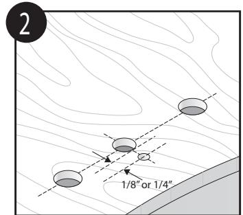
Drill the roll pin hole with a 7/32" drill. Position the roll pin hole 1/8" or 1/4" from the front edge of the spout hole depending on the spout that will be installed. (See Spout List)
