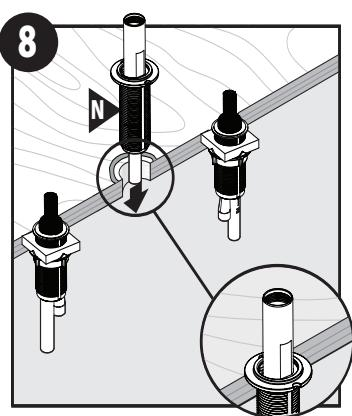
Place the assembled shank into the deck opening.
