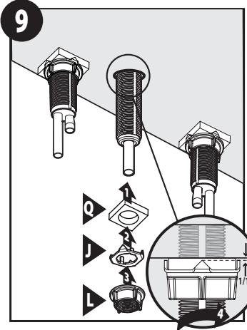
From the underside of the deck, set the black rubber washer (Q) on top of the locking washer (J) positioned with the points up. Tighten the mounting nut (L). Check roll pin location of mounting nut (F). Use pliers to secure nuts. **Tighten the nut so that the points of the metal washers are 1/16" maximum from the underside of the deck.**
