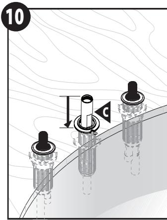
Slide the spout shank (C) to the lowest position. Shank height can be adjusted at spout installation.
