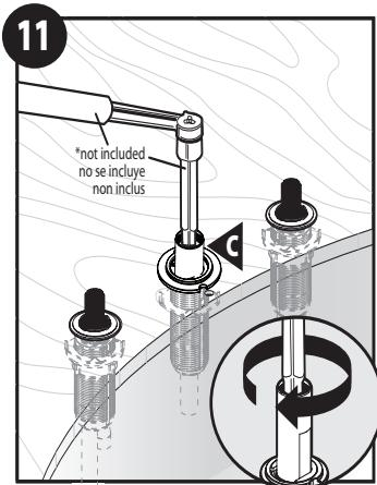
To secure the shank, use a 3/8" drive ratchet with a 6" extension (not included or 150313 tool). Tighten the expansion nut inside of the shank (C) by turning clockwise before pressure testing.
