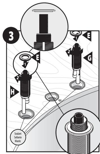
Thread the top mounting nuts (E) clockwise onto each valve (G) and (H) until they bottom out on the outer part of the valves. Apply a bead of sealant around all 3 holes.
