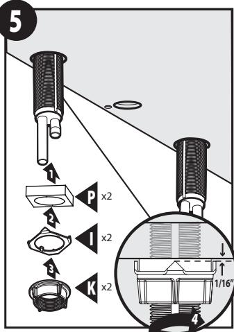
From the underside of the deck, set the black rubber washers (P) on top of the locking washers (I) positioned with the points up. The tabs on the washers will align with the groove in the valve body. Tighten the mounting nuts (K). Use pliers to secure nuts. **Tighten the nuts so that the points of the metal washers are 1/16" maximum from the underside of the deck.**
