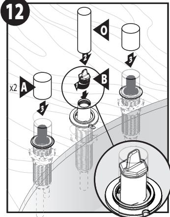
Thread in the test plug (B) and pressure test for leaks. Do not reuse test plug (B). NOTE: If pressure testing exceeds 125 psi, replace test plug (B) with brass test plug from Service Kit #100538. Slide on valve covers (A) and shank cover (O).
