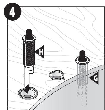
Position both valves (H) and (G) so the shorter legs (outlets) face in towards the spout.
