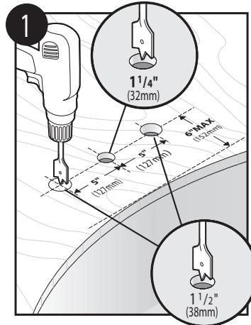
Drill holes for the valves and spout 5" minimum on center. Position the spout hole so that spout delivers the water to the desired place in the tub.
