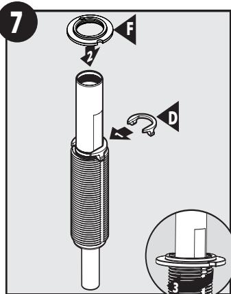
Slide the chrome clip (D) onto the flats of the shank as shown and slide down until tabs lock into the notches on the valve body. Thread the top mounting nut (F) onto the valve body over the clip. The nut secures the clip.
