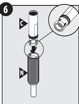
Check that the expansion nut is threaded into the bottom of the adjustable shank (C). Slide the adjustable shank (C) into the spout body (N) and position the shank so the flat sides are directly above the grooves.
