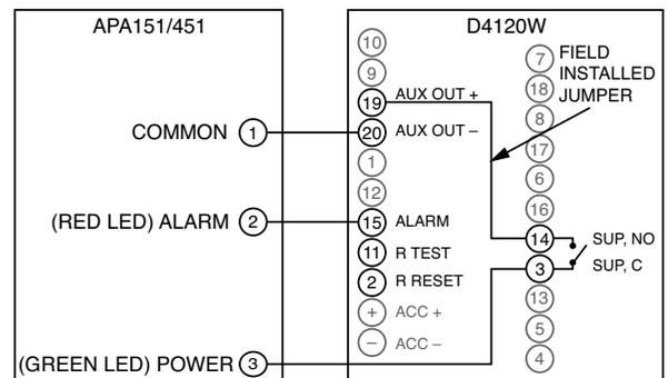
NOTE: WIRING DIAGRAM SHOWN IS FOR D4120W 4-WIRE DUCT SMOKE DETECTOR SYSTEM EQUIPPED WITHOUT A CONTROL PANEL. HO584-03
