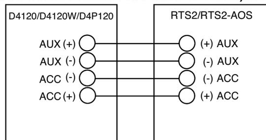
NOTE: If polarity of Acc. (+) and Acc. (-) are reversed, an Amber LED on sensor 2 of the duct smoke detector power board will exist indicating a trouble condition.
