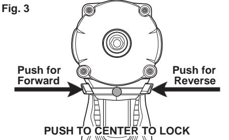
For **forward** (clockwise) rotation, push the control switch in the direction shown. Check the direction of rotation before use.
