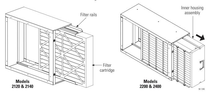
**5.** Align the assembled Upgrade Kit frame with the filter rails in the air cleaner housing and slide the frame completely into the air cleaner.
