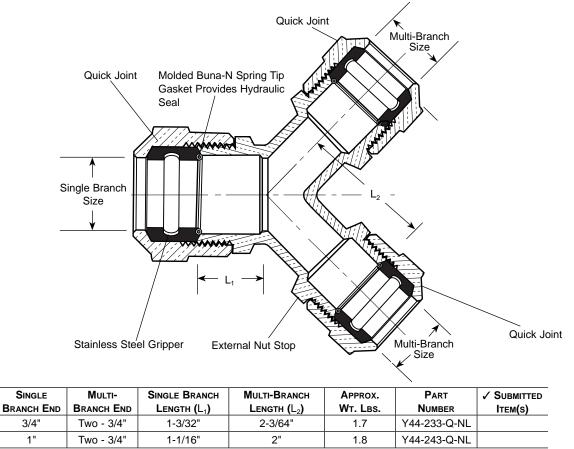
Note: Ford recommends insert stiffeners when using plastic pipe or tubing.
