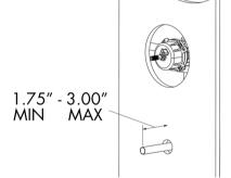
Slide spout (1) over exposed stub out pipe until flush to wall. Center the spout (1) on the wall and tighten set screw (2) from underneath with Allen wrench.
