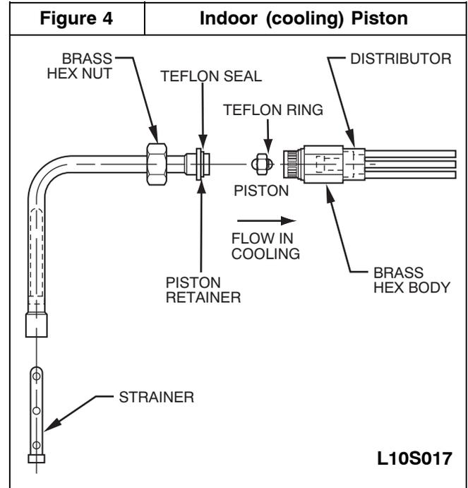
**Installing with Indoor Piston – cooling operation.**
