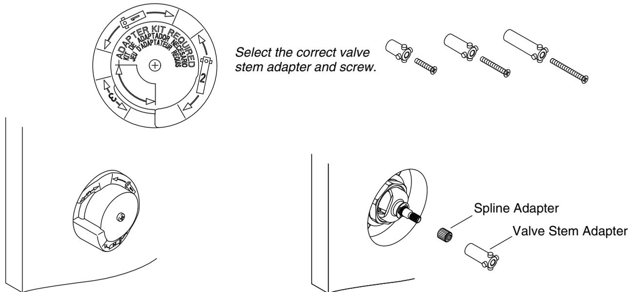
NOTE: Check the finished wall surface as related to the graphics on the plaster guard.
