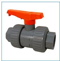
**Specifications UPC** Code 039923241900 Ball Valve Type **Connection Type** Universal (S & F) x Universal (S & F) 0.96 lb Weight Valve Size 3/4 **PVC** Material **Valve Operator** Direct Handle Description U45TB-E 3/4 TUBV EPDM PVC MOD-D eClass Classification PVC Sch 80 Ball Valves Color Dark Grey
