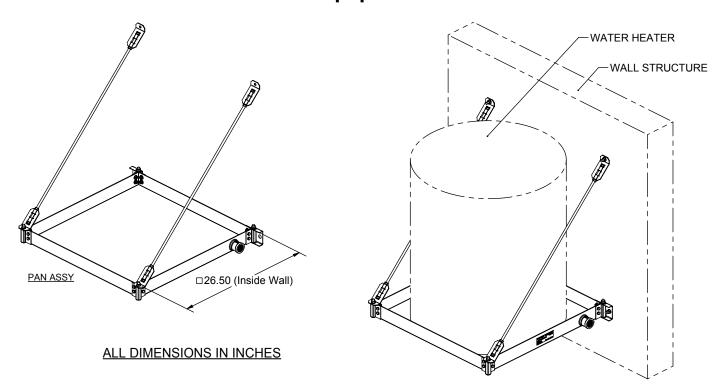
The Wall Mounted Equipment Platform is engineered to support water heaters up to 50 U.S. gallons (or other equipment up to 600 pounds total weight) mounted to a wall. This item also serves as a drain pan. See Installation Instructions for detail.
