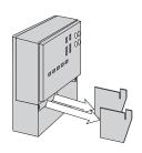
Remove the safety dividers from the wiring chamber by pulling them straight out of their grooves.
