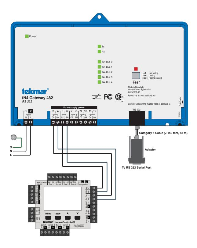
Refer to the D402 data brochure for a complete wiring schematic.
