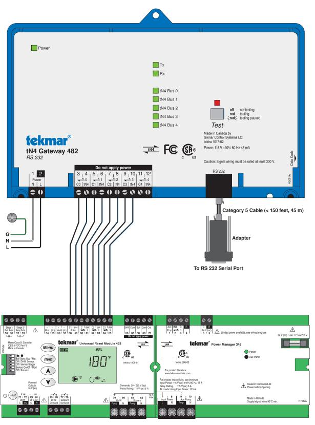
Refer to W423 and W345 wiring brochures for complete wiring schematics.
