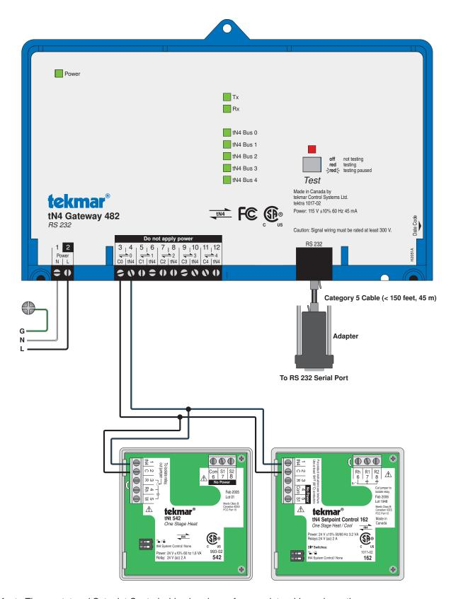
Refer to Thermostat and Setpoint Control wiring brochures for complete wiring schematic.
