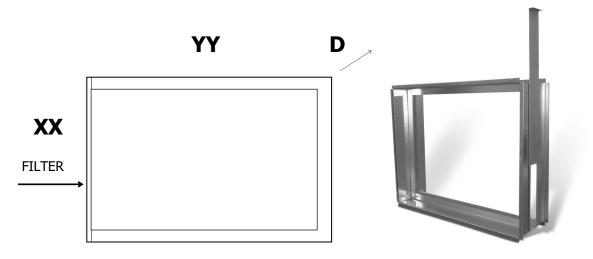
Depth of Frame Box is 2" greater than largest filter thickness (5" Filter = 7" Wide Frame Box)
