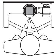
3. When the user steps away from the SOLIS® Sensor, the Sensor initiates an electrical signal that operates the Solenoid. This initiates the flushing cycle to flush the fixture. The Circuit then automatically resets and is ready for the next user.
