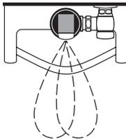
2. As the user enters the beam's effective range (15" to 30") the beam is reflected into the SOLIS® Scanner Window and transformed into a low voltage electrical circuit. Once activated, the Output Circuit continues in a "hold" mode for as long as the user remains within the effective range of the Sensor.
