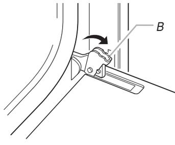
B. Oven door latch in unlocked position
