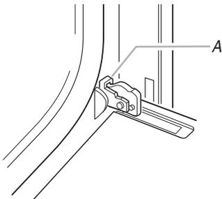
A. Oven door latch in locked position
