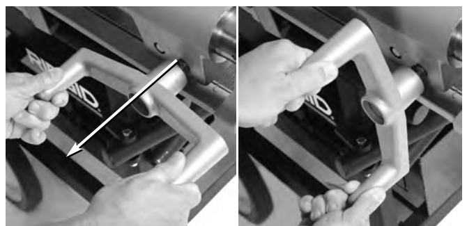
Figure 20 – Carriage Handwheel Adjustment
