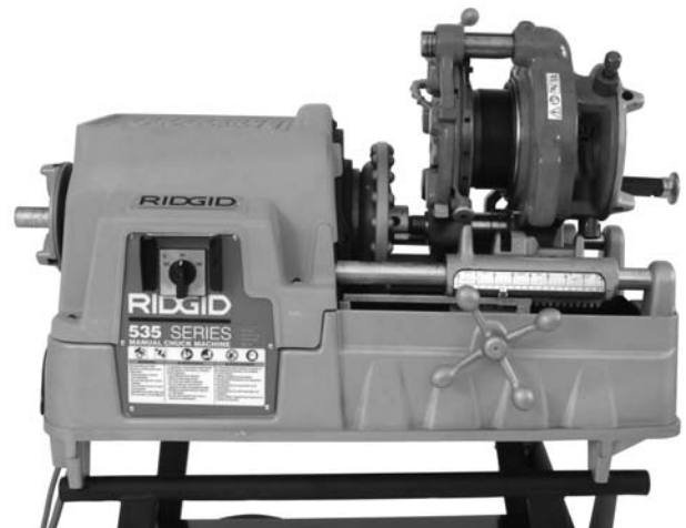
Figure 17 – Geared Threader Close-Coupled To 535
