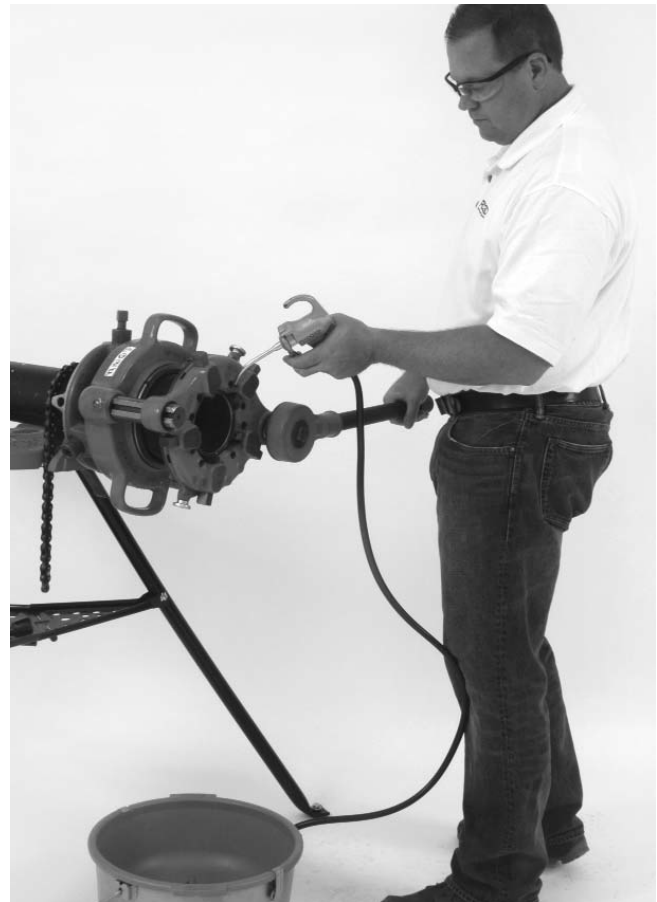
Figure 7 – D-1440 Ratchet Operation
