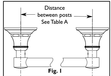
2. Drill hole(s) in wall at points marked using the appropriate drill size:
