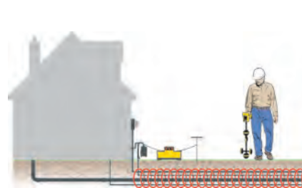
Direct connect to utility lines.
